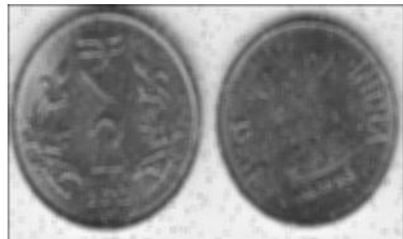
Figure.6 Mean filter used on Salt and pepper noise (Rohit Verma, and Jahid Ali, 2013)
